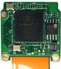
1. Using FPGA V main control chip of Altera and 28nm low power (LP) technology of the TSMC's, its total power consumption is 40% lower than Cyclone IV, 55% lower than the Cyclone III (while the competing products Basler uses cyclone III chip, and PointGrey uses Spartan-6 chip which has the same quality with Cyclone IV).
